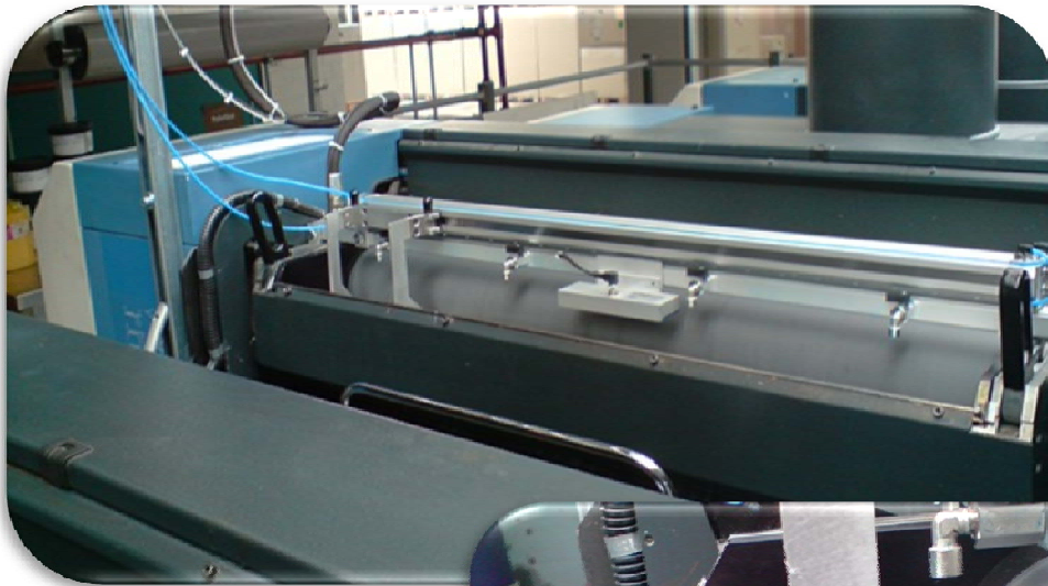
Ink agitator BIA-PSH with double scraper blade
