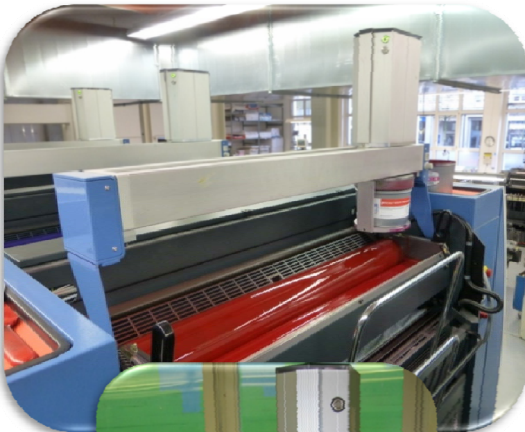
Automatic ink filling of the ink fountains out of standard 2,5kg cans. Version for UV plastic cans is also available.
