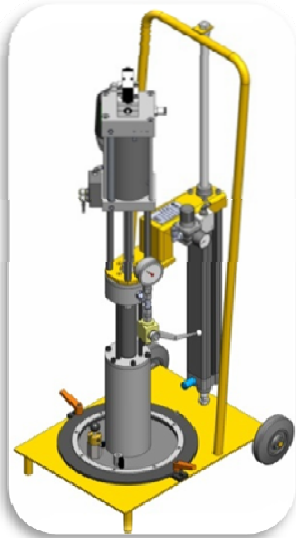
Pail can pump P100/113-25H Delivery/double stroke 113 cm 3 Pressure ratio 21 : 1
