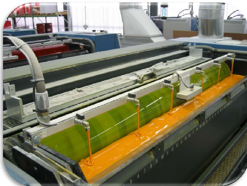
Ink leveler in filling position
