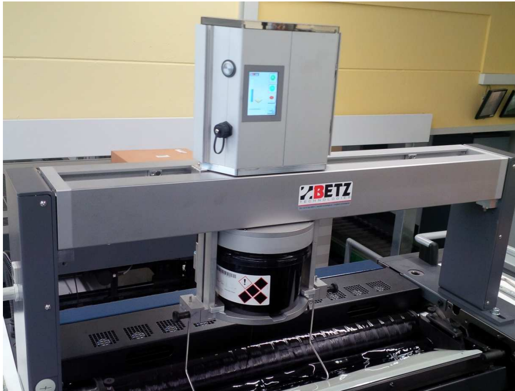
Pneumatically driven ink agitator BIA in connection with Ink leveller BLS
