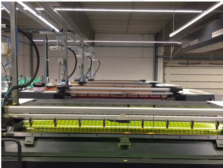
Pneumatically driven ink agitator BIA in connection with Ink leveller BLS
