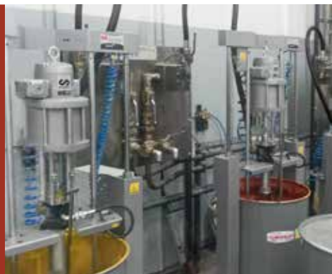
PM35 60:1 ratio Dynamic-Primer lubrication equipment pump package for dispensing heavy greases.
